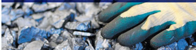
Multicrystalline silicon ingots are directionally solidified, under carefully controlled conditions, from molten, high purity polysilicon, in production systems designed and manufactured internally at the Group's facilities at Crystalox Limited, in the United Kingdom. During 2017 we will transition to purchasing ingots from an external supplier.
