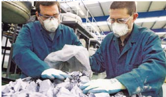
Crucibles are filled with high purity silicon
